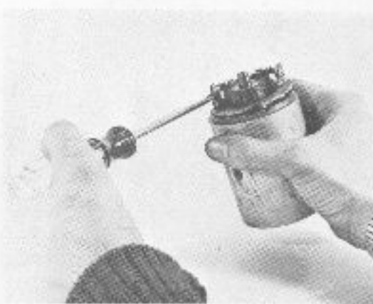
Disconnecting the brush leads
