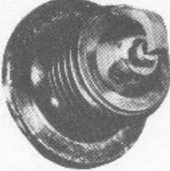
Splash-fouled: caused by installation of new plugs after a long-delayed tune-up
