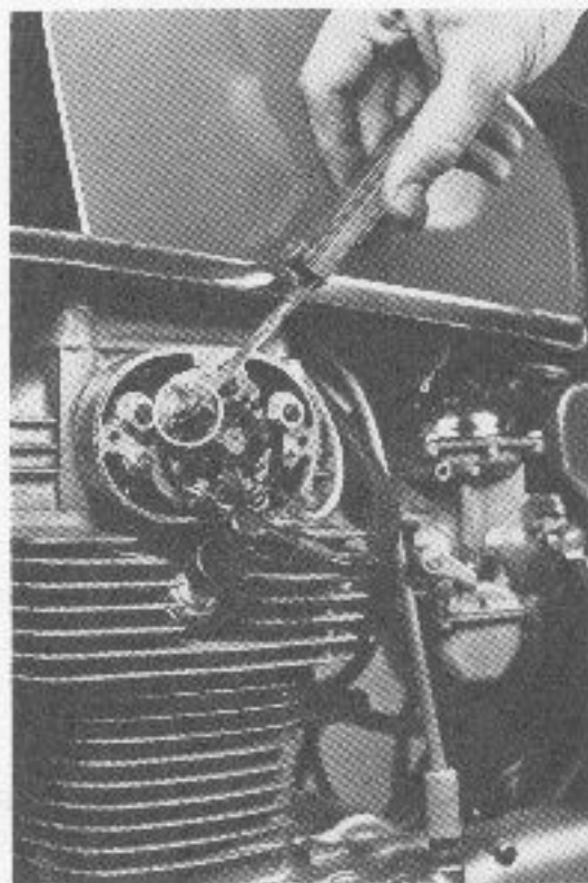
Checking point gap
