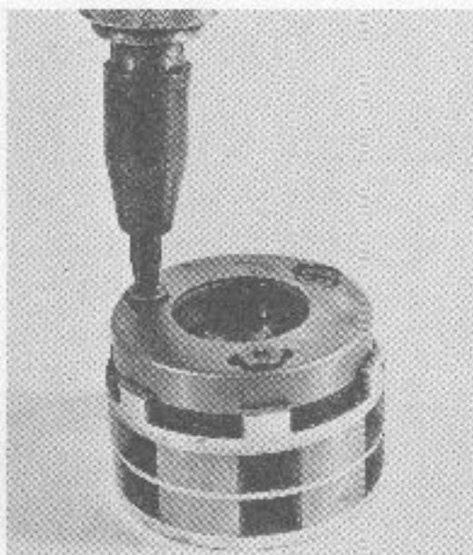
Removing the starter clutch from the alternator rotor
