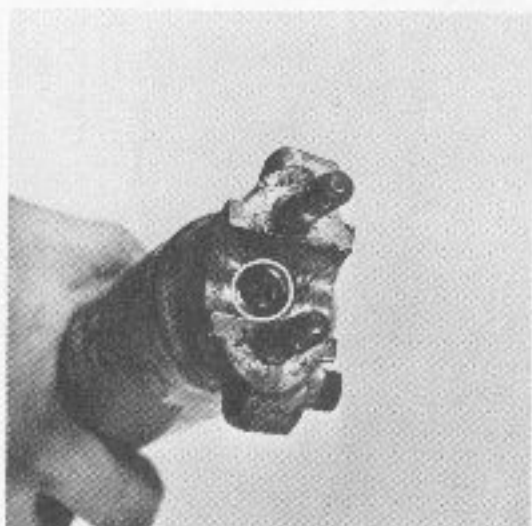
Slider screw must be removed with an impact driver
