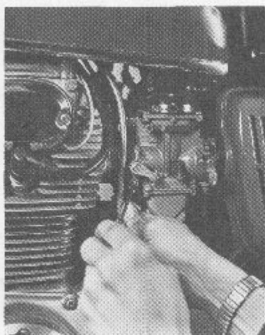
Setting the pilot screw
