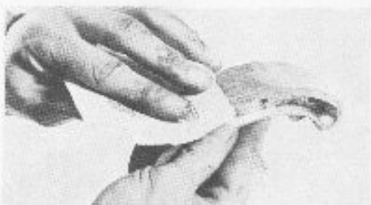
Sanding a brake lining
