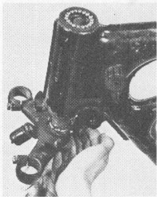
Removing the steering stem.
