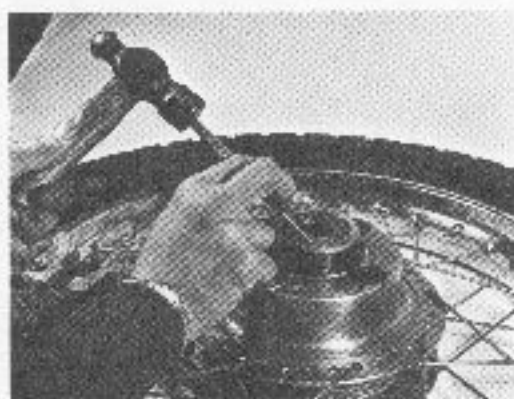
Removing bearing retainer (350 shown)
