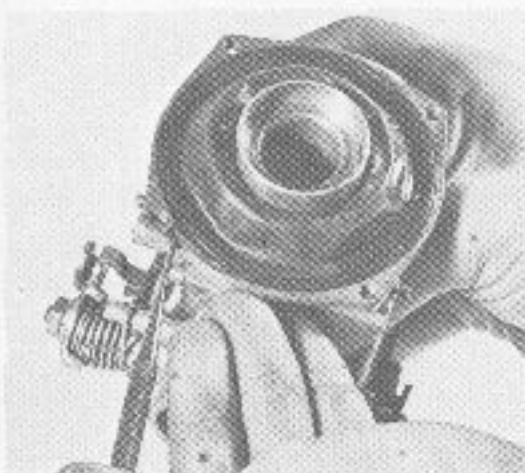
Fit the tab on the diaphragm into the slot in the body
