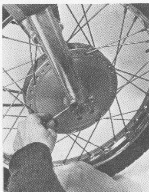
Removing the fork drain plug
