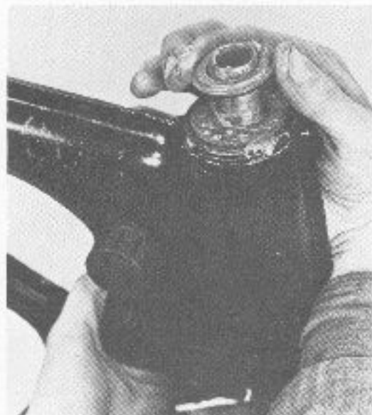
Installing the upper cone race
