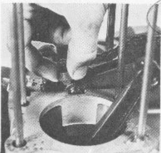
Installing the rubber roller pin inserts
