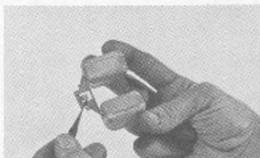
Bend the float tang to adjust float level
