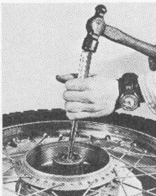
Removing wheel bearing
