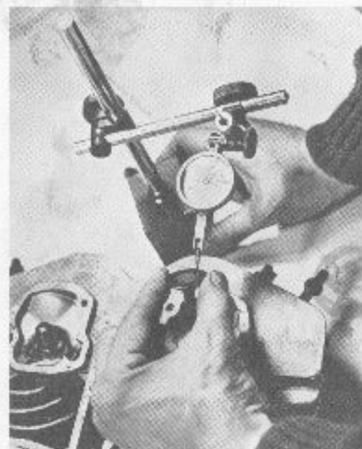
Checking for a worn valve guide
