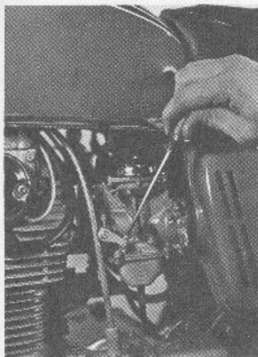
Adjusting the throttle stop screw (350)
