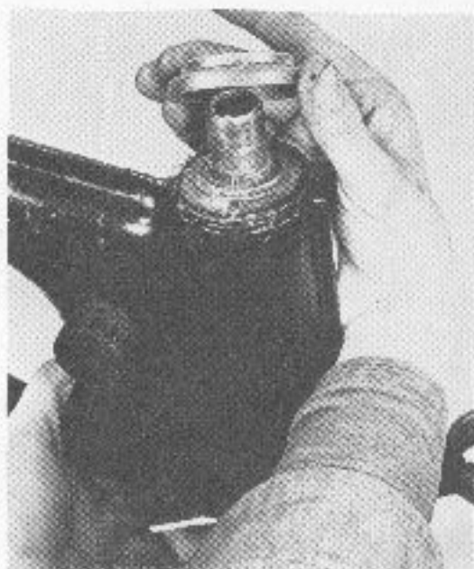
Removing the adjuster nut.
