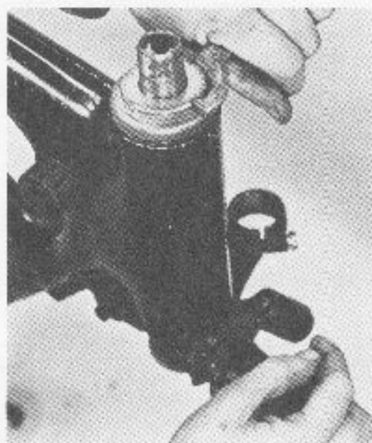
Adjusting the steering bearings with the Honda pin wrench.
