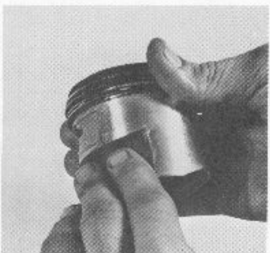
Removing score marks from the skirt with emery cloth: produce a crosshatch pattern when sanding.
