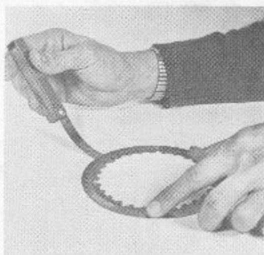
Checking a steel plate for warpage
