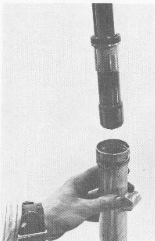
On early model fork, assemble the damper components on the inner tube and then insert the inner tube into the slider
