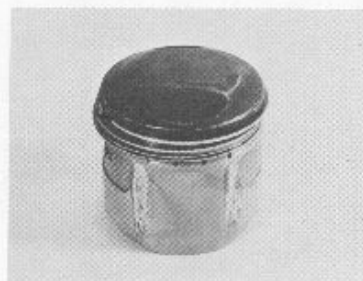
Scoring on this piston was caused by a seizure.
