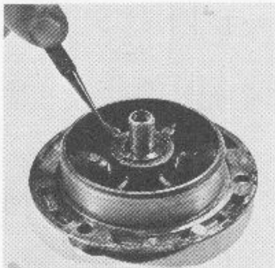
Checking oil guide operation.
