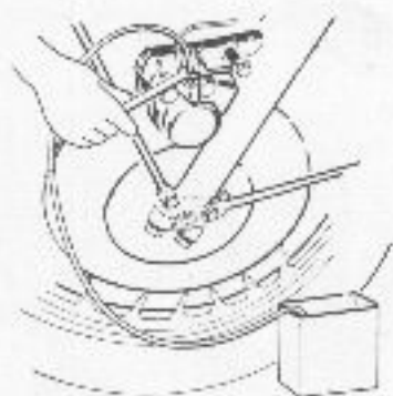
Bleeding the disc brake
