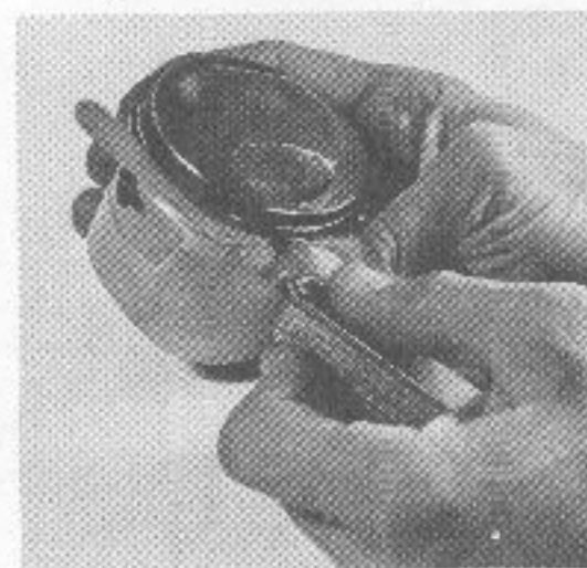
Checking ring side clearance
