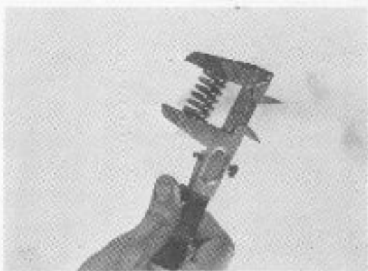
Measuring clutch spring free-length
