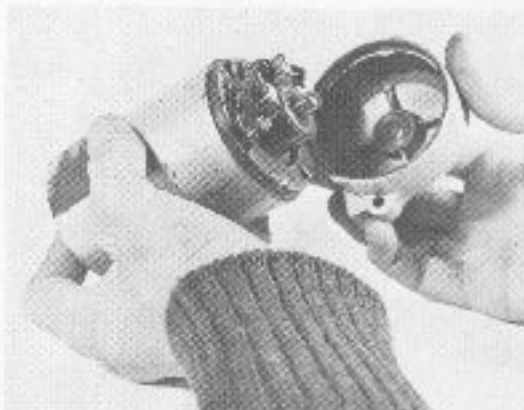
Removing the brush side end-plate
