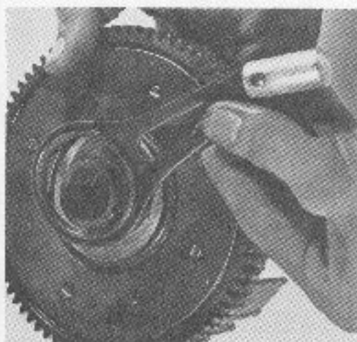
Removing the oil pump connecting rod
