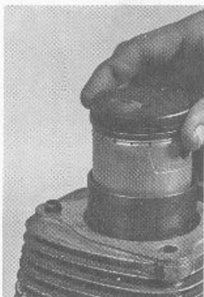
Square the ring in the bore with the bottom of the piston
