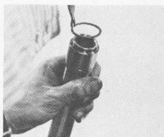
On early model forks, remove the circlip to remove the damper components
