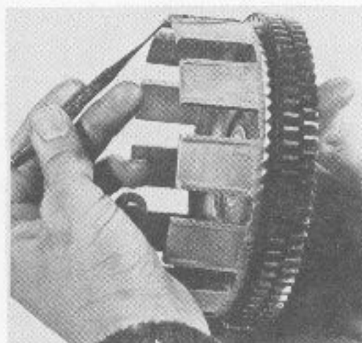
Check the clutch housing for indented wear caused by the plates
