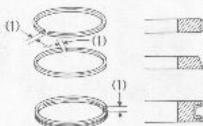
When installing the rings, space the end-gaps 120° apart (1); ring cross-sections show proper installation of 360 cc rings
