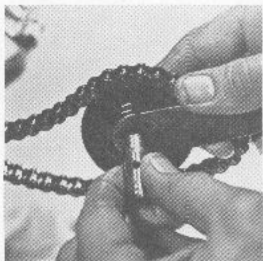
Removing the tensioner roller assembly
