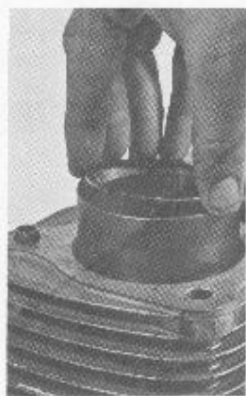
Insert each ring into the bottom of the bore to check ring end-gap
